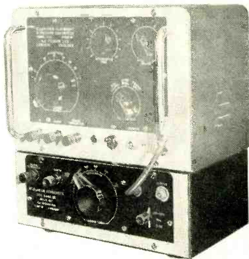
Band III convertor (below) for the type 1320 Cossor Tele-check swept-frequency oscillator (above).
