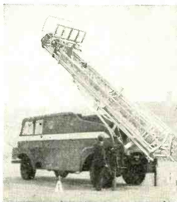
A PARABOLOID four feet in diameter is mounted on top of this 60-ft mobile extensible mast which the B.B.C. has recently introduced for television outside broadcasts. The aerial, which can be remotely rotated through 360°, can be adjusted to within \pm 1^\circ . When extended the mast is self supporting but provision is made for stay wires if needed.
