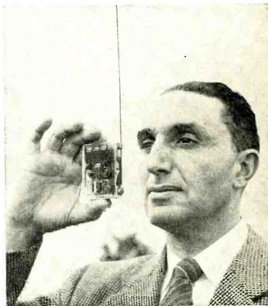
ONE way of solving the battery problem—but perhaps more suitable for nomadic Arabs than for stay-at-home Britons—is exemplified by this new transistor transmitter, which is powered entirely by sunlight through the medium of selenium cells. Built by Edward Keonjian (General Electric Company of America), it has a range of about 100ft.
